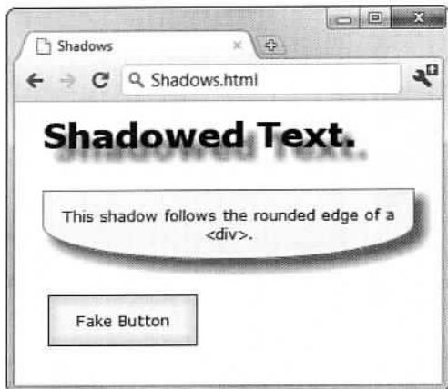
Figure 8-13: Shadows can make text float (top), boxes pop out (middle), or buttons look glowy (bottom).
